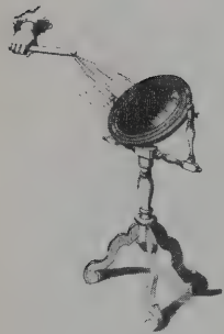
Small burning mirror used by 16th- and 17th-century natural scientists. From A Golden Thread , John Perlin, 1980 (out of print).
